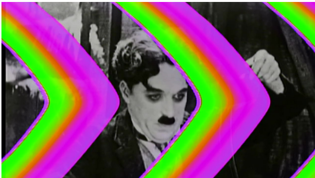
Burstless monochrome video input with AB set to AUTO or ON.
