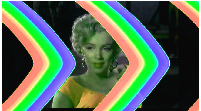
Colour video input with AB set to ON. NTSC Input becomes hue shifted.
